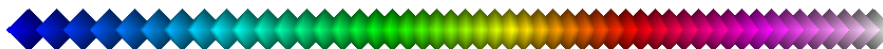
Figure 3.12: A line segment where the element nodes are marked with polygons. The mesh has 50 elements and thus 51 nodes.
