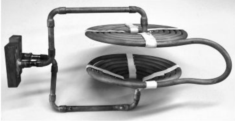
Device for electromagnetic levitation melting experiment
