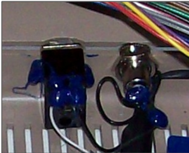
The Socket and switch affixed to the case.
